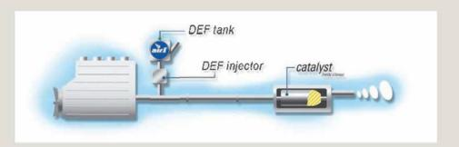
SCR technology is already proven to enable Heavy Diesel Vehicle engines to comply with Euro V legislation which took effect in 2008. Airl is the most efficient way to take full advantage of SCR technology and to meet EPA emission regulations.
